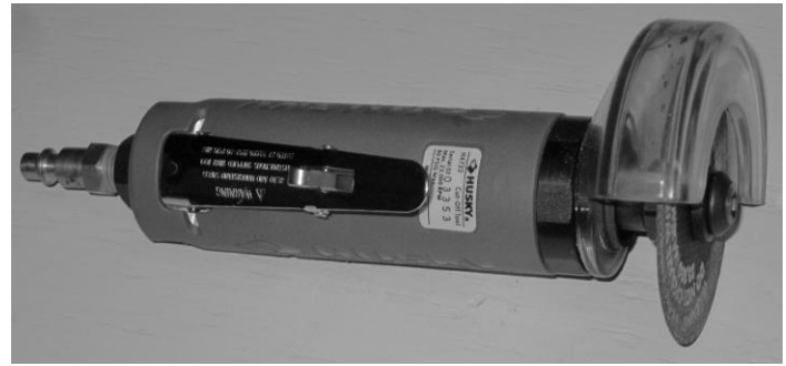
Figure 2. High speed cut off tool, air-powered 3" dia metal cut-off blade, abrasive.
